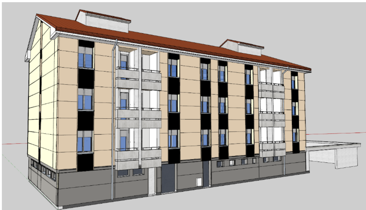
Figure 14: Panel distribution on frontal and side view (south and west façade)
