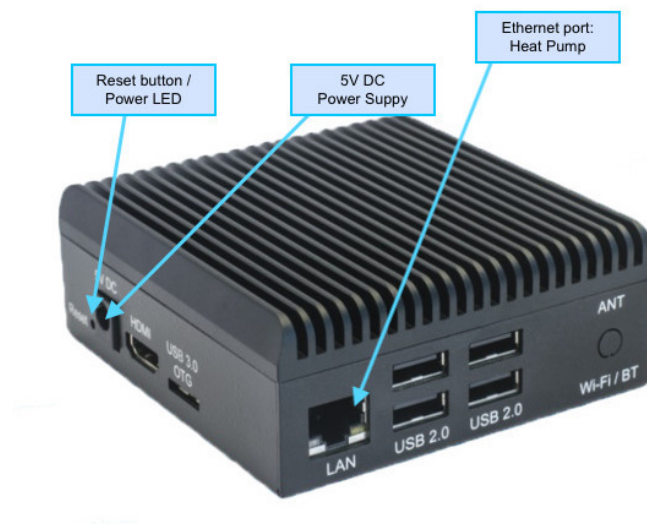
Fig. 27. Heat Pump Gateway installation details
